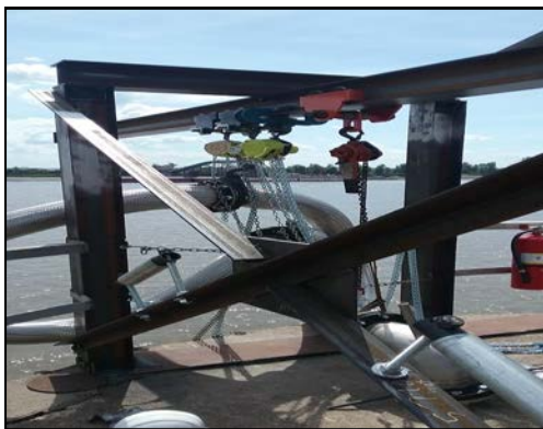
Above: Winch arrangement facilitates barge unloading. An improvised unloading system was approved to facilitate fuel transfers in the Port of St. Louis after Hurricane Harvey.
