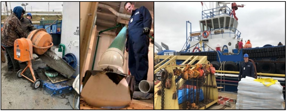
Above: An offshore towing vessel takes on ballast in the Western Rivers. In November, the Vessel Inspections Division witnessed an operation seldom seen on the Western Rivers. A seagoing towing vessel bound for San Juan, PR had 30 long tons of fixed cement ballast poured into its bilges to comply with its stability letter. The vessel also maintains a Load Line Certificate issued by the American Bureau of Shipping (ABS) therefore an ABS surveyor was also on board to witness the operation. The installation took several days to complete and to allow for the cement to properly cure.
